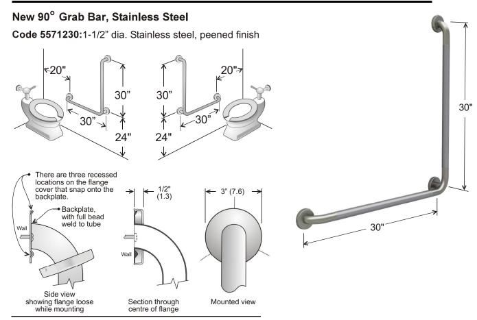
Concealed mounting screws, using snap flange.
