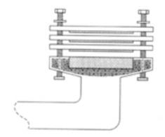
**Directions:** Ensure exiting flange is clean and place extension ring(s) on top of flange to raise flange to required height. Rings can be solvent welded or use a bead of caulk to secure rings together.
