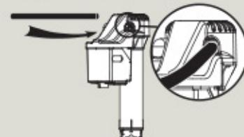
Tip: Run tube under warm water for easier install.
