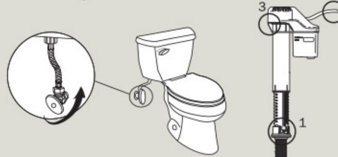
Congratulations! You have successfully installed your new fill valve. If hissing occurs, the flapper may be leaking. Shut off the water supply and let the toilet sit for an hour. If the water level drops, you likely need a new flapper. The Korky Ultra™ (100BP) is the best choice for most toilets with standard 2" flush valves. For large 3" flush valves, use the Korky 3060BP.
