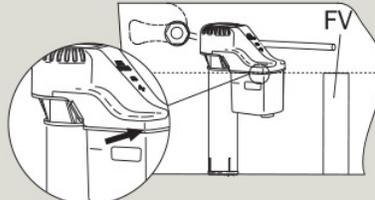
**c) Install mounting nut. Hand tighten only, beveled side up.**
