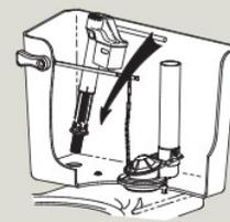
**3 a) Press down until corner of silver cover and top of flush valve (FV) line up.**
