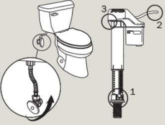
**c) Turn refill adjuster dial (D) clockwise to open.**
