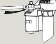
Tip: Run tube under warm water for easier install.
