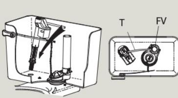
**b) Verify corner of silver cover and top of flush valve (FV) line up.**
