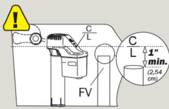
**b) Attach tube to flush valve (FV) with metal clip so water flows into flush valve. Trim tube if kink occurs.**
