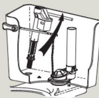
**c) Twist upper half of valve clockwise to lock (snap). Rib (R) lines up with pegs (P). Keep locked.**
