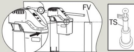
Tip: If tower style flush valve (TS), match fill valve water line to water line marked in tank (stain line).
