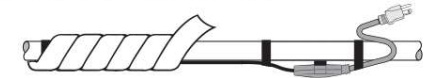
Automatic pipe heating cable on metal water pipe. (see 'Special Notes for Plastic Pipe' below).
