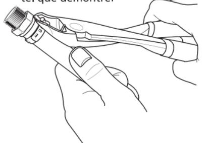
**NOTE: DO NOT USE THIS SURLOK TOOL TO REMOVE STAINLESS STEEL CLAMPS. ANY USE OTHER THAN INSTALLATION WILL VOID ANY AND ALL WARRANTIES.**
