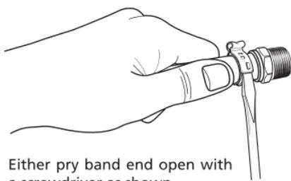
Either pry band end open with a screwdriver as shown...
