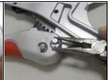
8. Fasten the body and handle with a dowel pin, turn upside down, fasten and complete set with Retaining ring.
