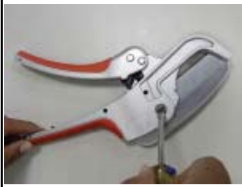
1. Unfasten the bolt in the back side with a slotted screwdriver
