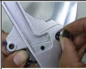
3. Fasten the blade by inserting a bolt
