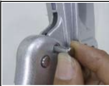
5. Pull out the dowel pin
