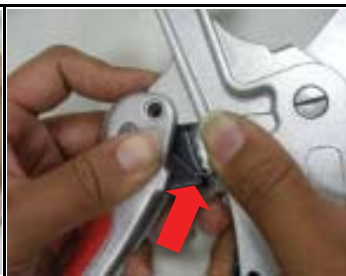
7. Match the sprocket with the teeth in the blade, then install the handle
