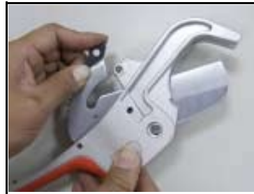
6. Disassemble the blade seat and replace the used blade with a new one
