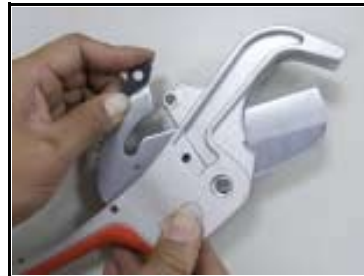
6. Disassemble the blade seat and replace the used blade with a new one
