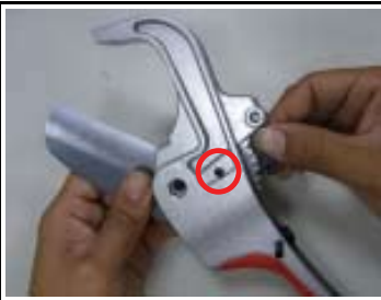
2. Install the blade and insert a spring pin inside the centre hole
