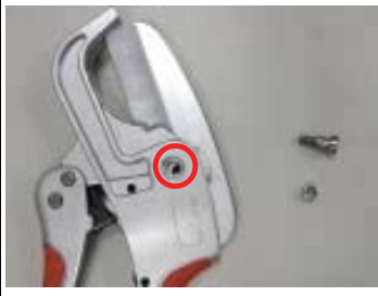
2. Take out the bolt and cap nut
