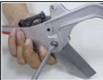
5. Turn upside down again and fasten the bolt with a slotted screwdriver
